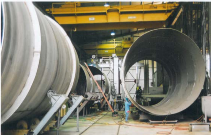
Stainless ASME Vessels (Lucedale Facility)
